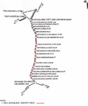
SOUTH WESTERN RAILWAY PROPOSED DOUBLING OF TRACK BETWEEN RAMANAGARAM AND MYSORE (NOT TO SCALE)
